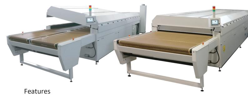
"Griff" is a tunnel oven with high air circulation. The gas heating has been chosen to reduce energy costs.
